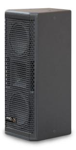
**Energy, compactness and lightness** are taken to the limit to achieve this amazing multipurpose system, as shows its Power Handling of 450 RMS / 900 W program / 1800 W peak and Maximum SPL peak of 128 dB in a compact and lightweight body of: 548x235x240mm and 12,4 Kg. Using CNC construction of 15mm made from birch wood plated on the exterior to ensure the maximum soundness.
