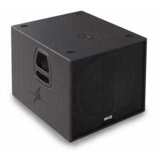
A super compact sub and an excellent bass reinforcement for all the systems of the IT / IT-A Series and M / MA Series thanks to its relationship between performance, size and weight. IT 115 F owns a Power Handling of 600 W RMS / 1200 W program / 2400 W peak, an Average Sensitivity of 99 dB and Maximum SPL of 131 dB, in a compact CNC construction of 15mm made from birch wood plated on the exterior, with measures 480x505x605mm and 32 Kg of weight.
