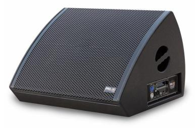
**ST 212** is **simply the best monitor system solution** thanks to its Power Handling of 1100 W RMS / 2200 W program / 4400 W peak. Average Sensitivity of 102 dB and Maximum SPL peak of 138 dB, super compact size (450x698x565) and light weight (33,3 Kg), using CNC construction of 18-15mm made from birch wood plated on the exterior.
