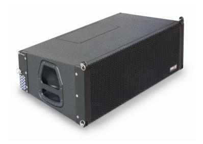
The most powerful, compact and versatile Line Array system of its rank, as evidenced by its high power handling (700 W RMS, program of 1400 W / 2800 W peak), compact size and weight (HxWxD: 280 x 735 x 465mm, 33,7 Kg) and its comprehensive and symmetric coverage of 120º at the horizontal plane without secondary lobes over the entire frequency range.
