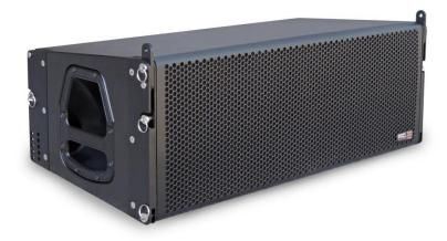
The New GT 2X10 L.A. is a new Line Array component of the GT Series family. GT 2X10 L.A. presents an impressive ratio between high performance and compact size, a Power Handling of 900 W RMS / program of 1800 W / 3600 W peak. A Maximum SPL peak of 135 dB (one unit) / 138 dB (four units), in a compact body with measures: (HxWxD); 291x811x385,5mm and 34,9 Kg of weight are just some examples of it.
