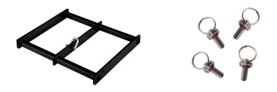
**Flight rigging pack composed by:** one (1) lightweight steel frame (with captive guide and links) + four (4) connection pin locks + one (1) shackle. To elevate up a total of 16 units **GT 2X8 L.A.** or **GTA 2X8 L.A.**
