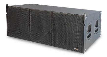
**Power, precision and compactness taken to the limit** to originate the most potent Line Array system of the **GT - GTA Series**. Generating a Power Handling of 2500 W RMS / 5000 W program / 10000 W peak and a Maximum SPL peak of 139 dB (one unit) / 142 dB (four units). All of this with the most compact and robust CNC construction of 18mm made in birch plywood plated on the exterior, instead the use of less resistant materials which don't guarantee the maximum safety.
