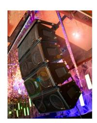
Flight hardware inserted to the cabinet with different angulation grades. Built in specially reinforced steel to ensure maximum safety.
