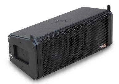
The perfect example of advanced high-end engineering thanks to its Power Handling of 450 W RMS / programme of 900 W / 1800 W peak, Average Sensitivity of 99 dB and Maximum SPL peak of 131 dB (one unit) and 134 dB (four units) in a super compact and lightweight body of 235x570x240mm and 17,6 Kg. Using CNC construction of 15mm made from birch wood plated on the exterior. Always respecting our high quality construction philosophy.
