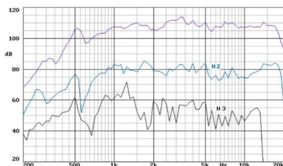
Note: on axis frequency response measured with 2 waveguides coupled to a 90° X 5° horn in an anechoic chamber, 1 w @ 1 m.
