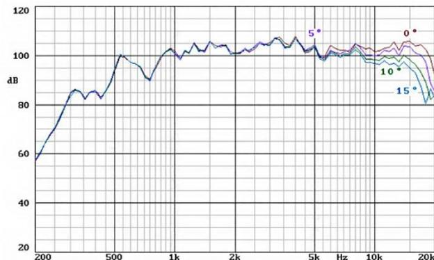
**Notes:** dispersion measured with two waveguides coupled to a 90° x 5° horn in anechoic chamber, 1w @ 2m.
