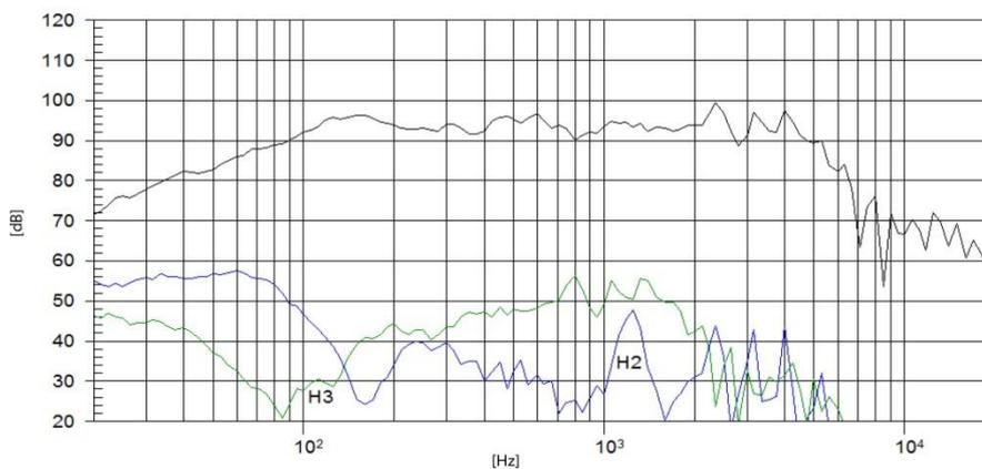
Note: On axis frequency response measured with loudspeaker standing on infinite baffle in anechoic chamber, 1W @ 1m
