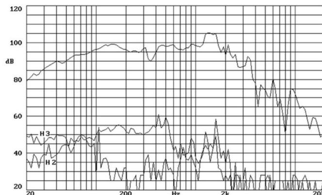
Note: On axis frequency response measured with loudspeaker standing on infinite baffle in anechoic chamber, 2.83v @ 1m
