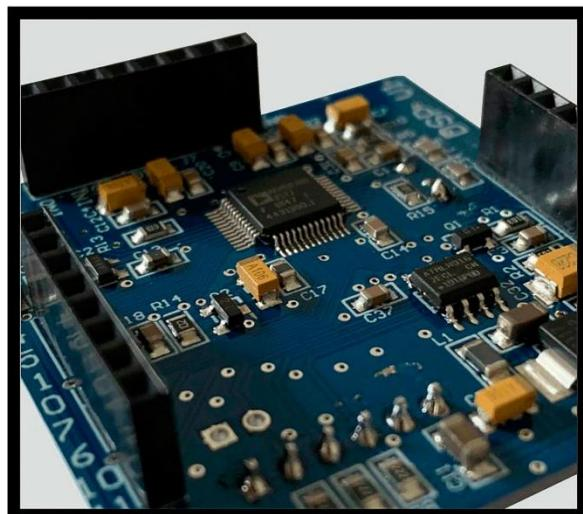
[EN] **IT-A 118 B** incorporates a new Class-D amplification module with 2 channels of 1\*1000w for Low + 1\*600w for SAT, with voltage selector. 96kHz DSP Processor, 24 bit with 3 factory presets. Speakon output for SAT in order to amplify itself and another passive unit **IT 1M6 i, IT 1M6 L.A. IT 2M6 i, IT 112 PA, i 403, i 803, M 10, or M 12**, which allows making configurations.
