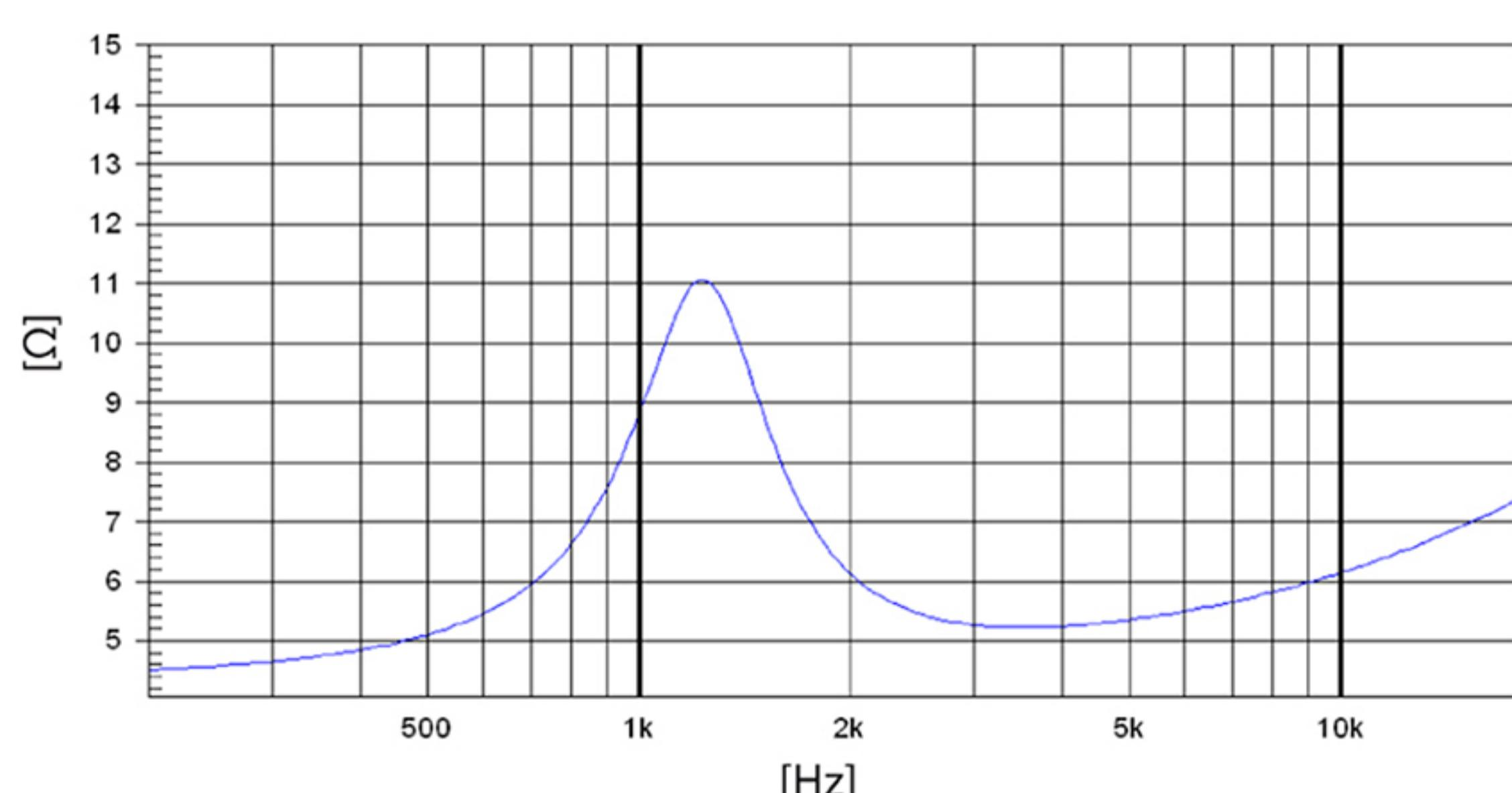
Note: Electrical impedance measured coupled to GT 2X15 L.A. horn
