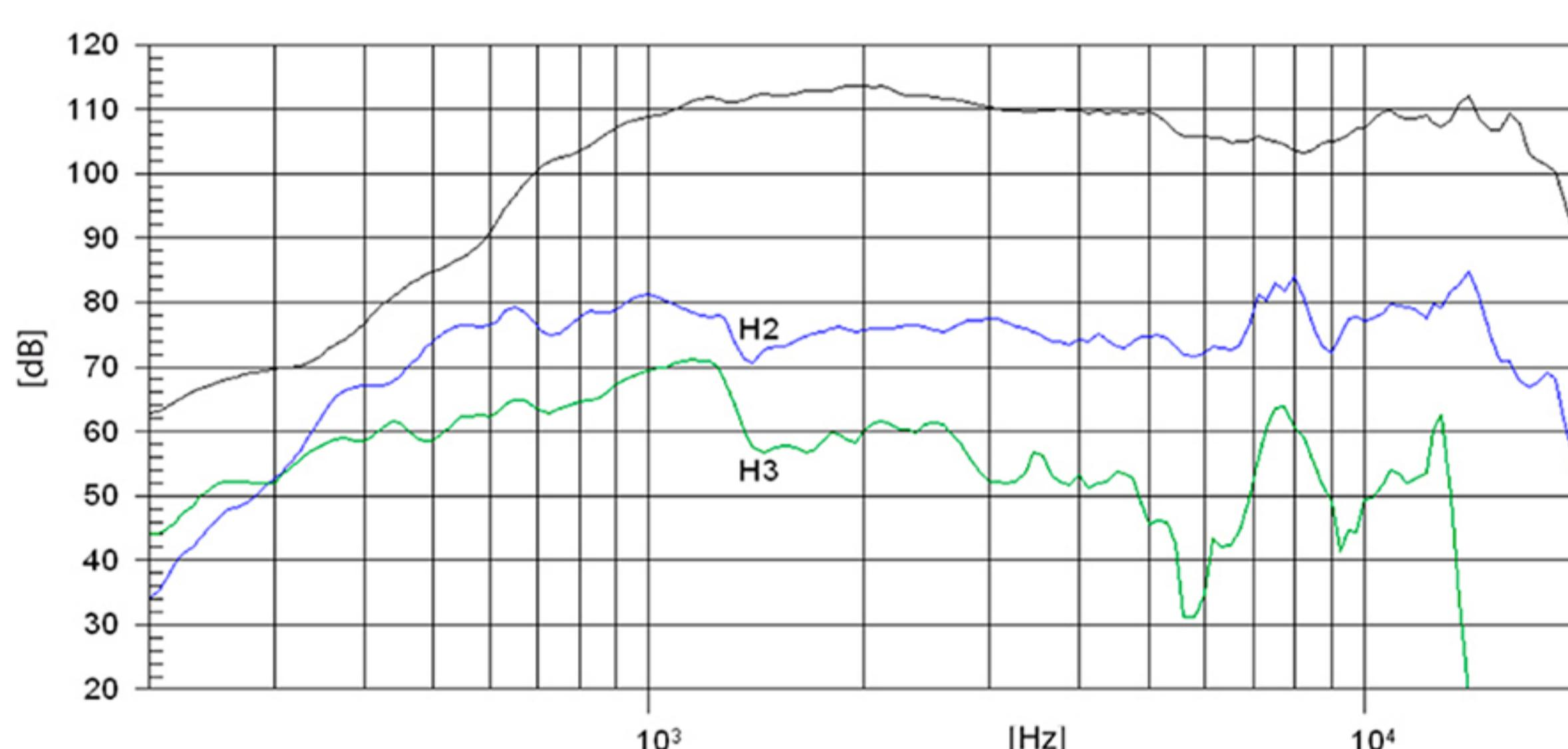
Note: on axis frequency response measured coupled to GT 2X15 L.A. horn in anechoic chamber, 2,83 v @ 1m
