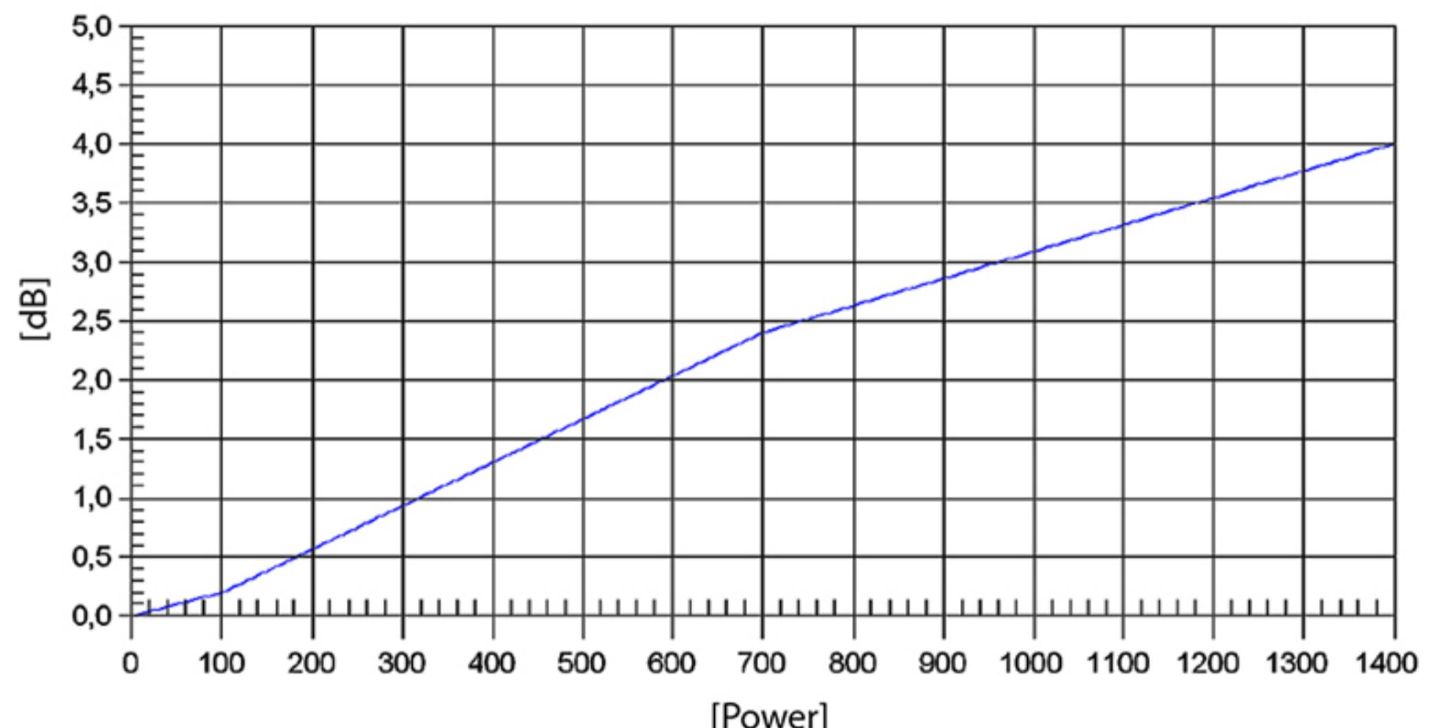
Note: Power compression losses were calculated after 5 minutes period applying a pink noise signal filtered between 25 and 200 Hz.
