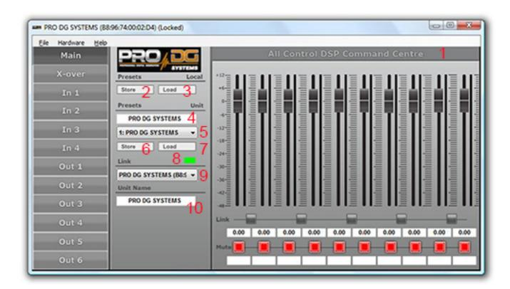
At this section you can make adjustments to the Input and Output Gain (1) (four inputs and six outputs for: PRO 26 loudspeaker processor, one input and two outputs for: GT 1.2 H / V, one input and three outputs for: GT 2.5 - GT 4.0 and GT 5.0).
