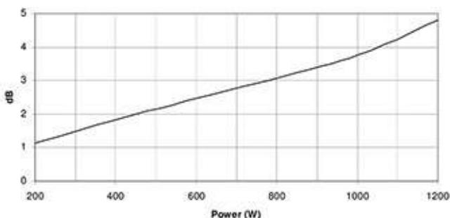
Note: Power Compression Losses were calculated after 5 minutes period applying a pink noise signal filtered between 40 and 200 Hz.
