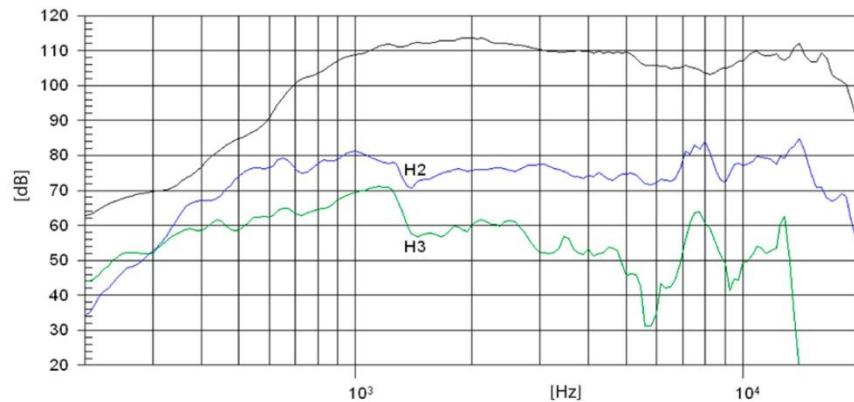
**Note:** On axis frequency response measured coupled to IT-A 112 P.A. horn in anechoic chamber 2,83 v @ 1m.
