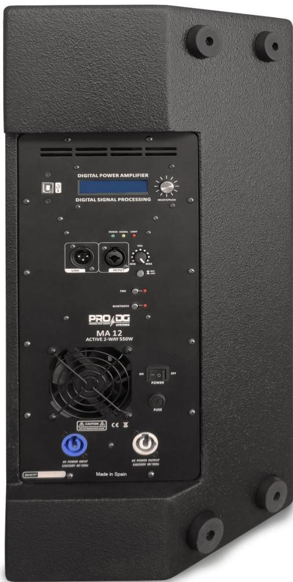
[EN] MA 12 incorporates a new Class-D amplification module with voltage selector. 96kHz DSP Processor, 24 bit with 3 factory presets. ON/OFF switch, volume control, Bluetooth ON/OFF switch, TWS switch, DSP management switch + LCD display for presets selection
