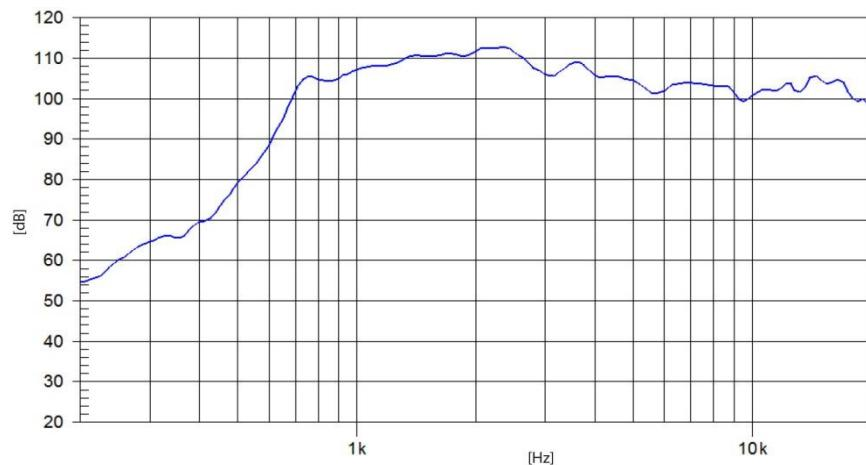
**Note:** On axis frequency response measured coupled to MA 12 horn in anechoic chamber 1W @ 1m.
