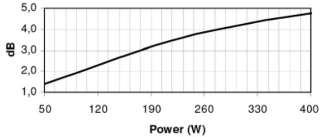
Note: These losses are calculated from a five minutes AES power test applying band limited pink noise (25 - 1200 Hz). The loudspeaker is free-air standing.
