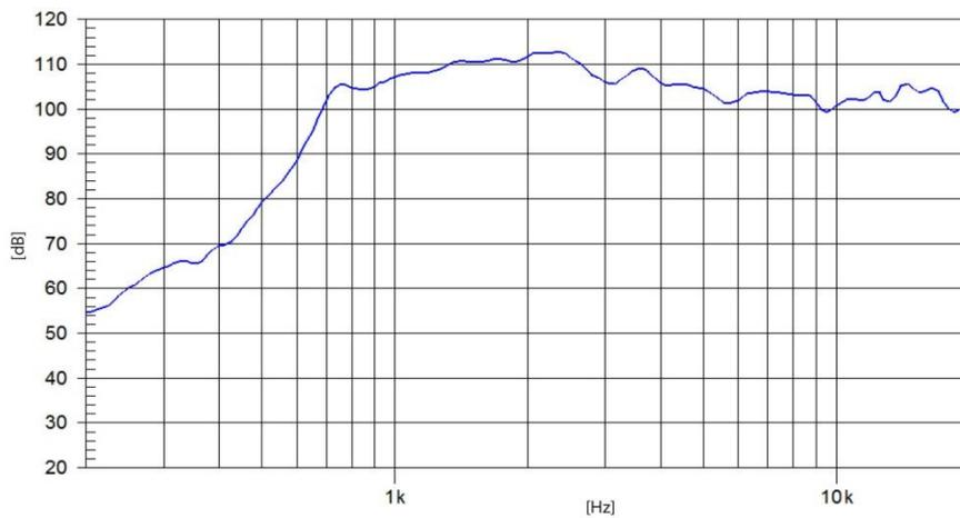
**Note:** On axis frequency response measured coupled to M 15 horn in anechoic chamber 1W @ 1m.
