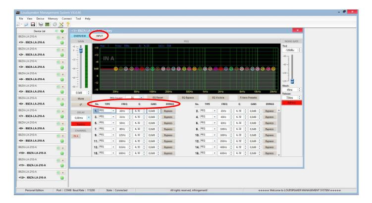
On the left of the menu, you can manually modify Gain, Mute, Delay, Bypass and input channel selection.
