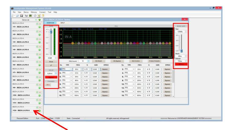
To apply changes to any of the units connected to the *ProDGnet* network, simply click on the desired unit.
