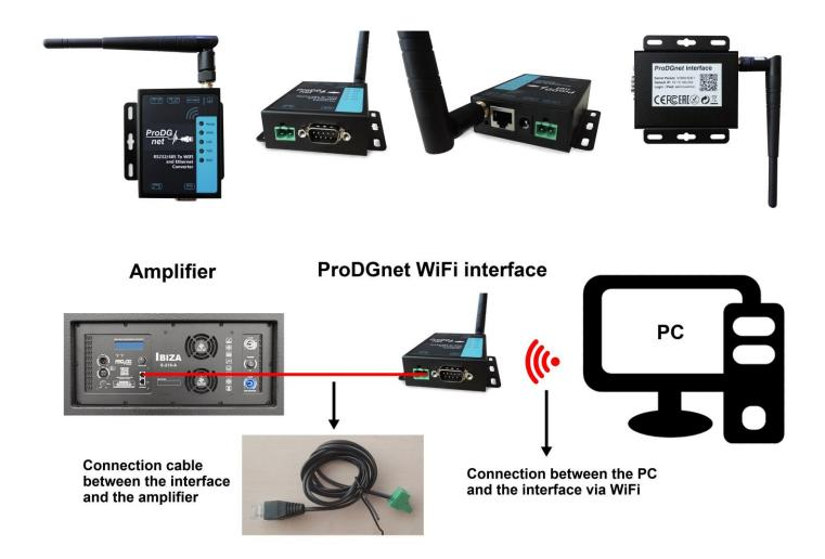
Both options work via RS485 protocol, allowing you to connect the DSP module housed in the amplifier to your PC.
